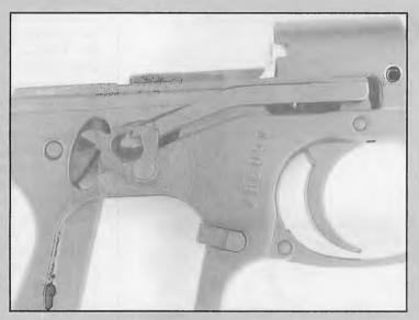
In the double-action mode, a pull on the trigger will draw the trigger bar forward. This rotates the sear forward on its axis pin, causing the hammer-cocking bent to be drawn forward and up, thus raising the automatic safety tumbler out of the hammer's path and rotating the hammer on its axis pin to compress the hammer spring. As the sear slips out of the cocking bent, the hammer falls.
